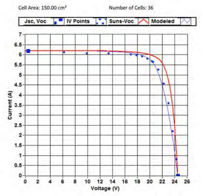
$V_{oc} = 24.4807 \text{ V}$   $I_{mp} = 5.64 \text{ A}$   $I_{sc} = 6.20 \text{ A}$   $V_{mp} = 20.45 \text{ V}$   $I_{sc} = 6.20 \text{ A/cm}^2$   $I_{mp} = 115.37 \text{ W}$  Fill Factor = 76.03 % Efficiency = 17.10 %  $I_{sc} = 0.26 \text{ Ohms}$   $I_{sc} = 0.26 \text{ Ohms}$   $I_{sc} = 0.26 \text{ Ohms}$
