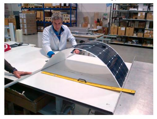
After the bending EL and Flash test have been repeated.
