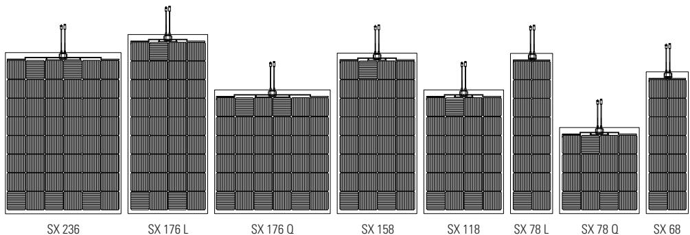
In the SX series the monocrystalline solar cells are electrically connected using ultra-thin copper wires that form a very fine mesh on the cell surface, resulting in thousands of contact connected points. This alternative to the standard bus-bar method allows a higher module power and increases the energy yield. A technology optimally suited to flexible modules, thanks to its intrinsic insensitivity to micro-cracks, that are the most common cause of energy loss in solar modules.
